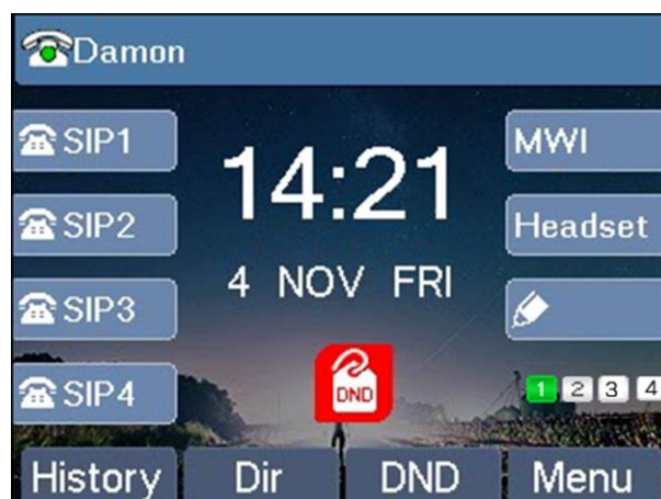
Figure 57 - DND Enabled on All Lines
